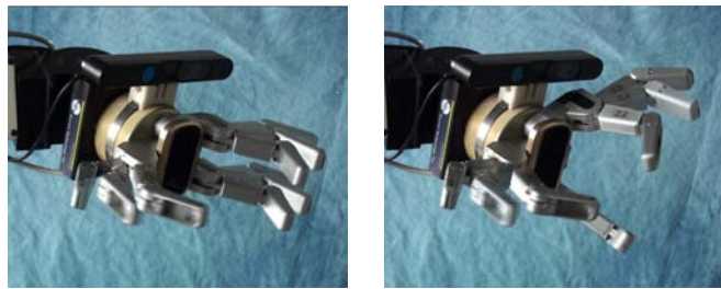
Fig. 1: The motion of two different preshapes of the Barrett Hand. To find suitable grasps we search for structure that is shaped complementarily.
