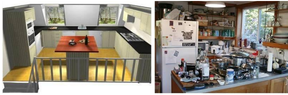
Fig. 2. Researchers often assume that a priori models, such as the CAD model of the kitchen on the left, are available. In practice, those models are usually difficult to obtain. Also, such environments are constantly changing and look more like the kitchen on the right.
