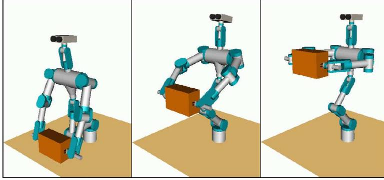
Figure 1: Manipulation and Posture Behaviors: a sequence of three snapshots from the dynamic simulation of a 24-degree-of-freedom humanoid system, whose motion is generated from simple manipulation and posture behaviors.
