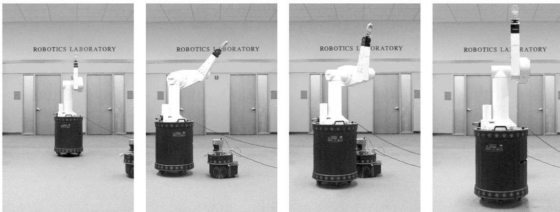
Figure 8: Demonstrating task-consistent obstacle avoidance with the Stanford Robotic Platform. The end-effector performs a straight-line motion, while the base avoids the obstacle, which is perceived using a laser range finder.
