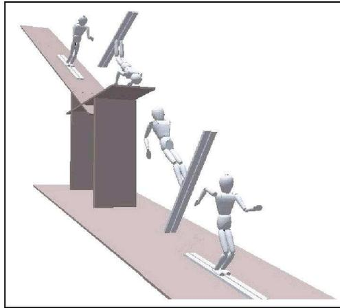
Figure 4: The image shows intermediate snapshots of a motion during a dynamic simulation involving contacts and impulses between an articulated body and its environment. The sliding motion and subsequent jump and landing are dynamically simulated in interactive time.
