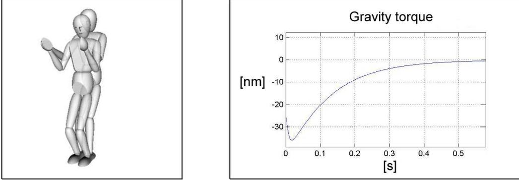
Figure 3: The robot minimizes gravity torque using postures: the task involves three operational points associated with the arms and the head while the posture motion requires the knees to minimize joint gravity torques. The starting posture has the knees of the humanoid bent. Upon activation the posture control straightens the knees to minimize gravity torques as shown in the data graph on the right.
