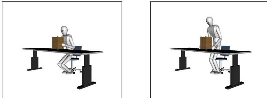
Figure 5: These two images show the motion of a humanoid robot combining task and posture constraints. Operational points at the hands are used to define the manipulation task, while another operational point on the hip permits to specify the rising behavior of the torso. Posture energies are employed to yield a natural-looking overall motion.
