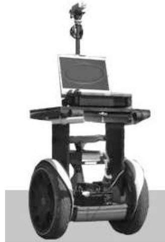
Fig. 2. The UMass Segway RMP, the subject of our previous work [36], is a robotic autonomous agent that can act as a network participant to improve performance in disruption-tolerant networks. Other platforms include robotic airborne vehicles [8] and underwater mobile robots [13], [14], [38], [34].
