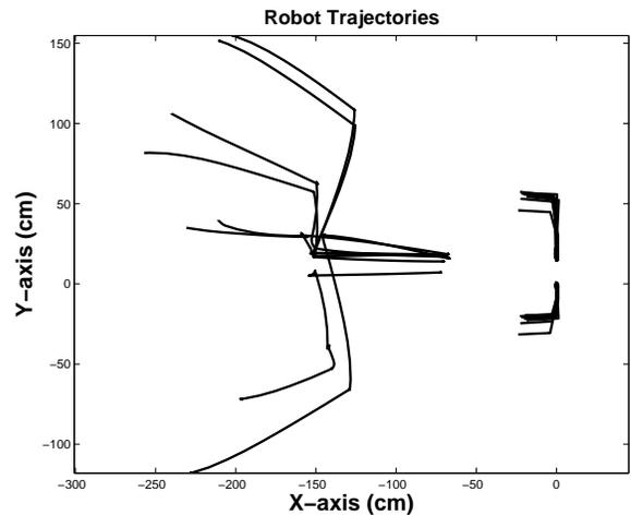
Fig. 6. The trajectories taken by Robonaut during the eight experimental trials. The “lightning-bolt” trajectories on the left side are the trajectories taken by the mobile base. The “L”-shaped trajectories on the right are the paths taken by Robonaut’s two palms.
