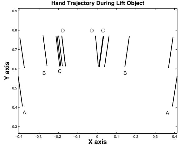
Fig. 4. An example of the trajectory taken by Robonaut's two palms as they grasp the sample box. After starting at configuration "A," the two palms reach toward the object toward configuration "B." Next, the robot executes guarded move and a compliance controllers that move the palms to configurations "C" and "D," respectively.
