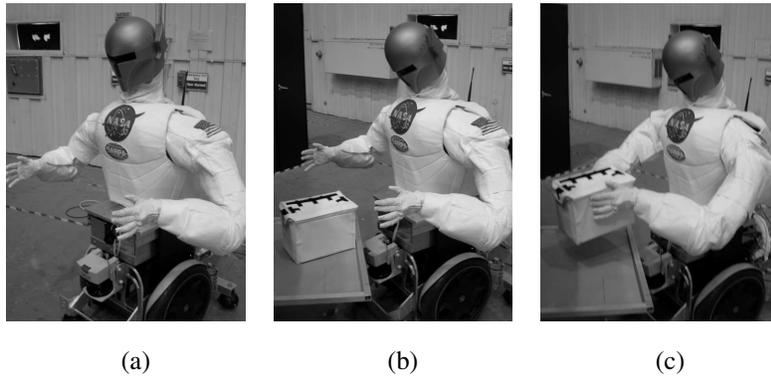
Fig. 5. Illustration of Robonaut completing the move-to-grasp task in the Robonaut-SCOUT field study.
