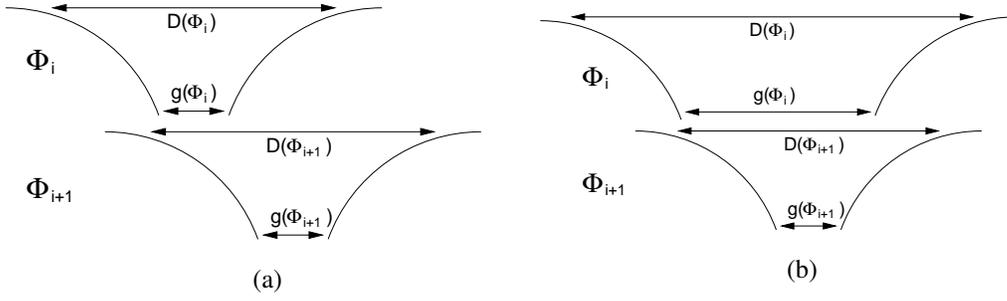
Fig. 1. Controller funneling, (a), compared with controller refinement, (b).
