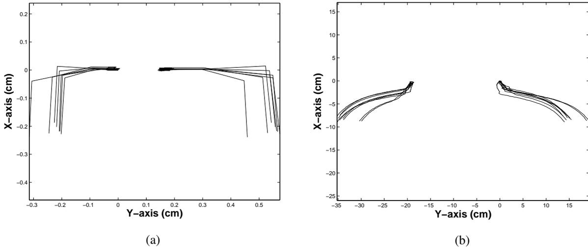
Fig. 8. The trajectory taken by Robonaut's two palms when executing the sequential control sequence, (a), compared with the parallelized control sequence, (b).
