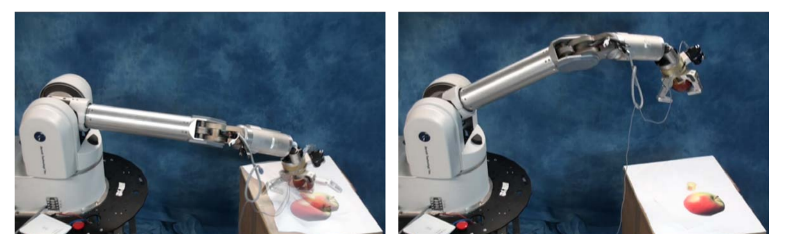
Execution of the spherical grasp controller using visual feedback.
