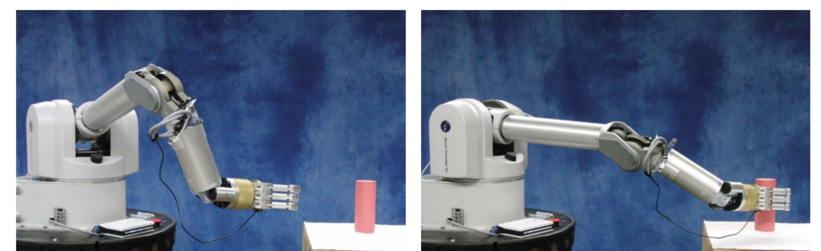
Execution of the cylindrical grasp controller using visual feedback.
