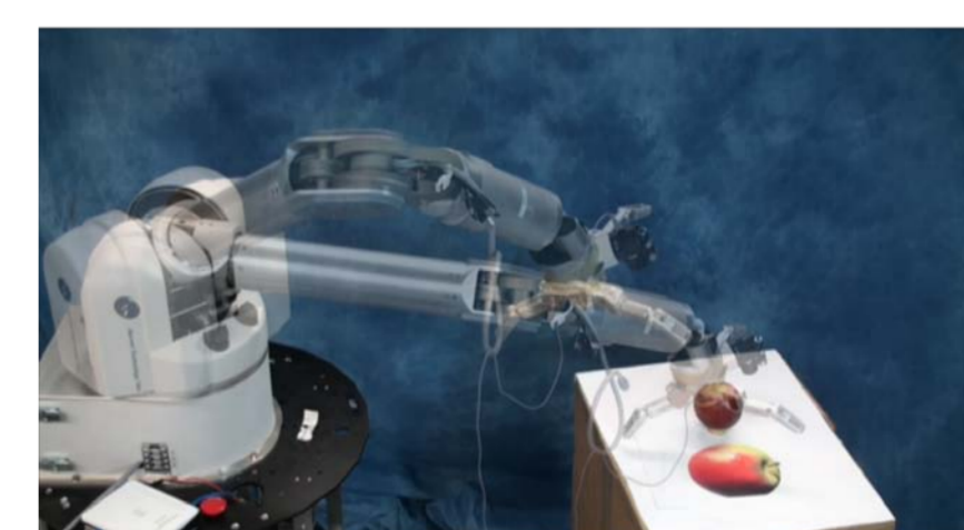
Execution of the cylindrical grasp controller using visual feedback.
