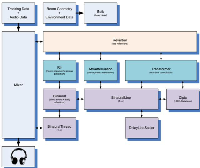
Fig. 3. Structure of the 3D sound-field synthesis module
