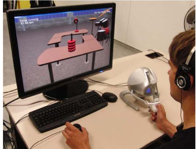
Fig. 5. Experimental setup of the table-top setup using the Novint falcon as a haptic interface in combination with a 3D-connexion Spacenavigator in order to exploit a large workspace
