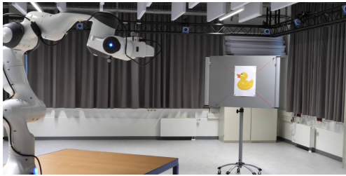
(a) Robot directed at a target in a motion capture system
