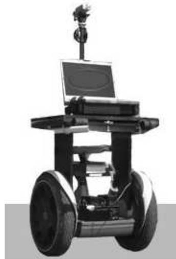
Figure 1: The UMass Segway Robotic Transporter [21]
